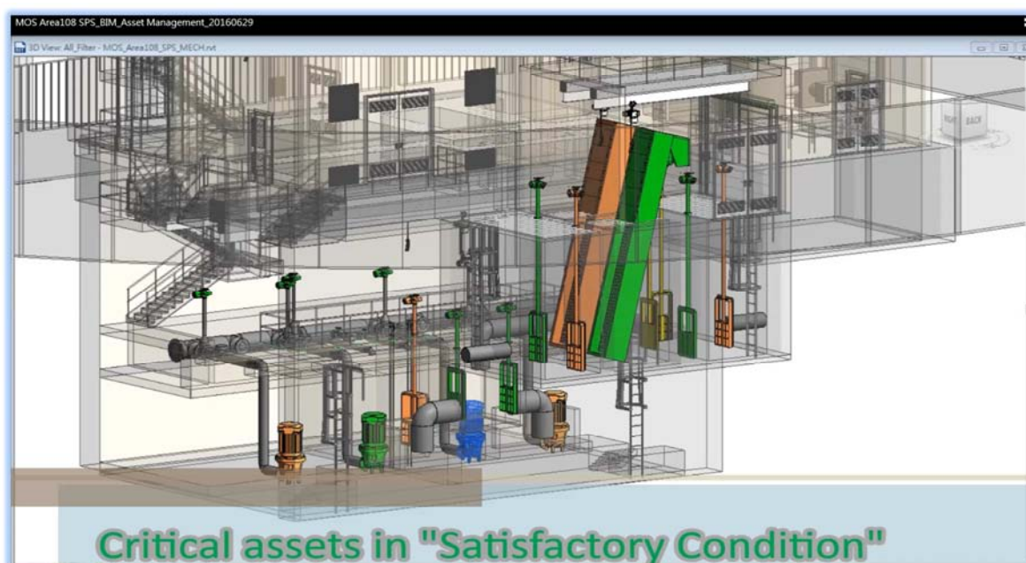
Figure 14. Color-coded asset health index in BIM model.
